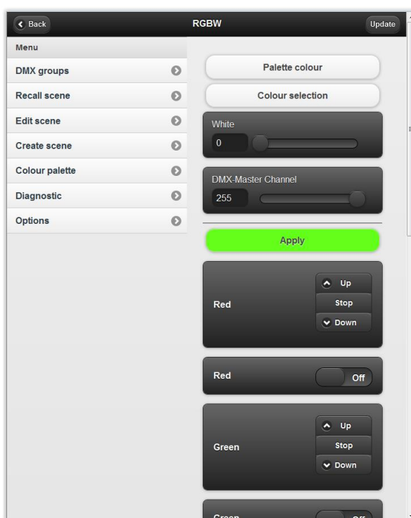
Fig. 4-35: Control of an RGBW group
